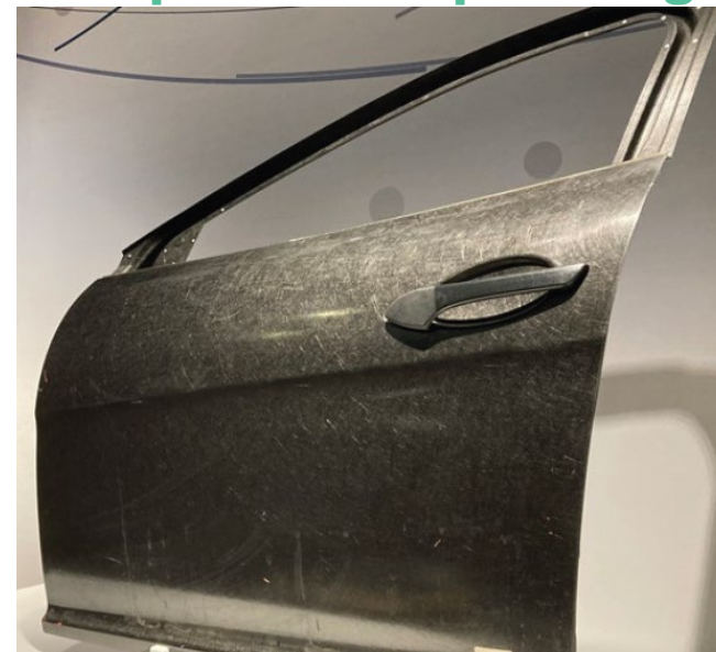
rCF reinforced Elium thermoplastic automotive door panel prototype (Recotrans project – courtesy of Gestamp)
