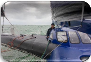
Recycled Elium (95% content): fairing & roof
