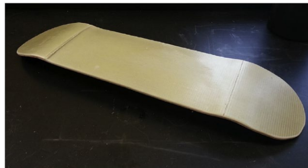
Fig. 10. A prototypical skateboard fabricated in part by thermoforming an Elium/glass fiber test panel as reinforcement.
