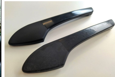
Door handle: recycled compound of 50% r-ABS and 50% composite CF of GF/Elium®
